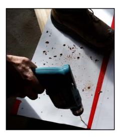
E. Once all holes are drilled, use a skill saw or table saw to cut the board to match the outer edge of the paper template to ensure accuracy when creating pattern repeat for the tactile indicator surface.
