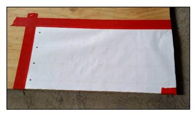
C. Use a hole punch to mark the areas to be drilled for the Bar or Dome template ensuring an accurate hole when drilling.
